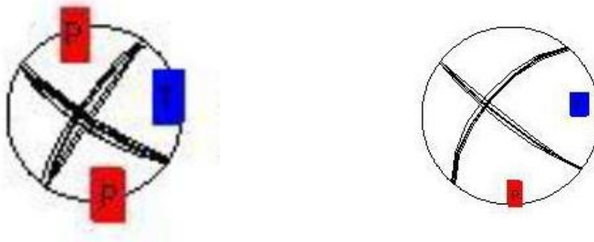
Figure 8. Test of stability of the focal mechanism of the main shock (left) and its largest aftershock (right) by repeatedly remove of stations (jackknifing). For each removal, a complete space–time grid search and least-squares MT calculations was done. As seen on the nodal planes, the responses are stable.
