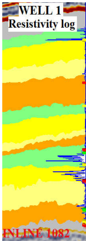
Figure 20. Resistivity log in Well 1
